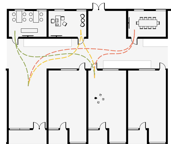
The new south wing is designed to create flexible space between classrooms, offices, study rooms, and labs.
