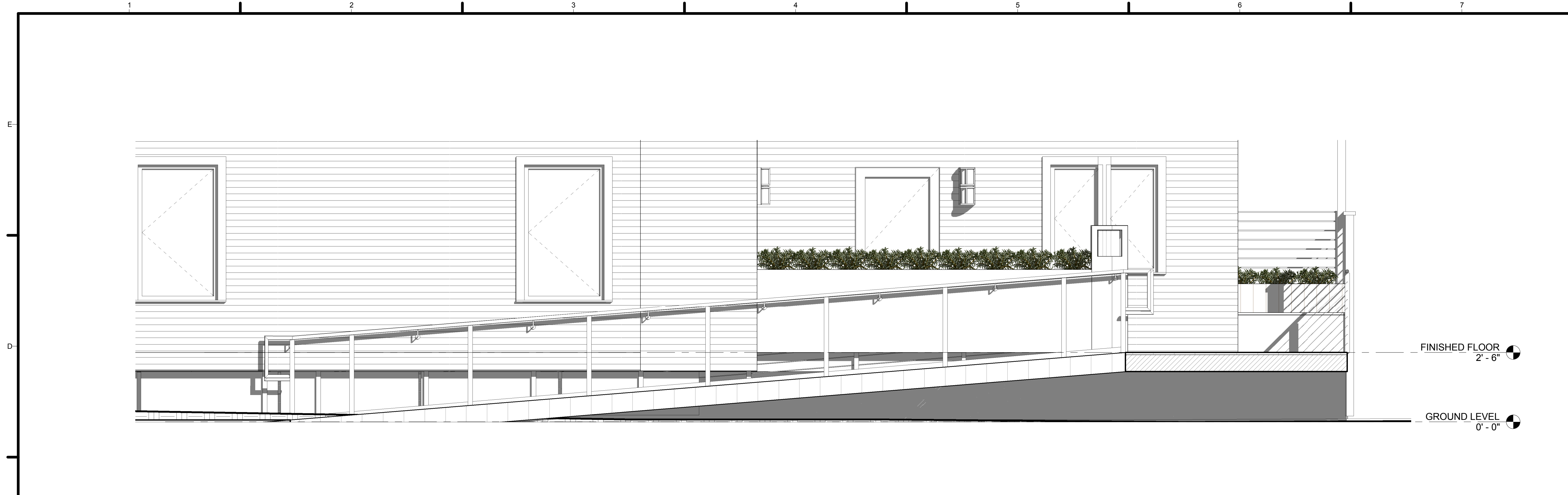
① RAMP SECTION - SOUTH VIEW 1/2" = 1'-0"
