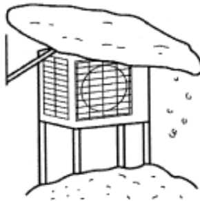
Figure 1: construction of canopy and pedestal
