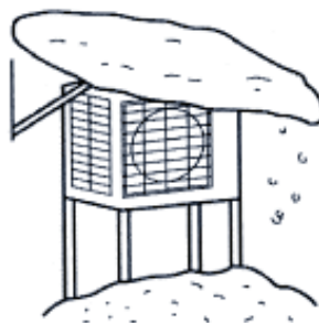
Figure 1: construction of canopy and pedestal
