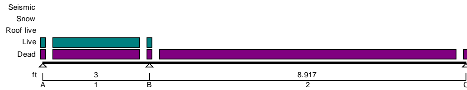
Load Combination 11 (shown in proportion)
