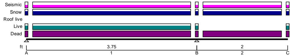
Load Combination 13 (shown in proportion)
