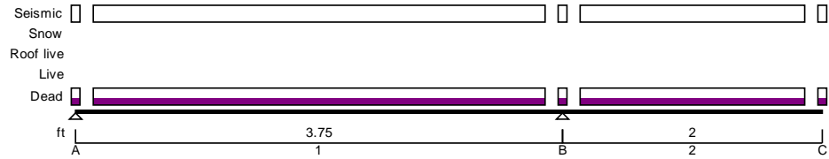
Load Combination 10 (shown in proportion)
