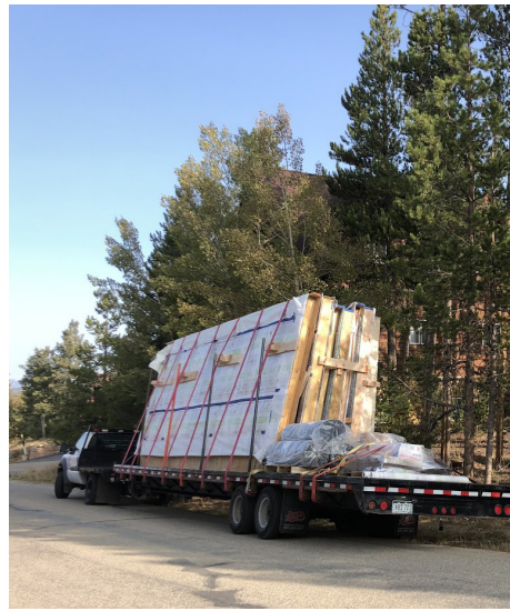
Figure 7: SPARC House panels on truck
