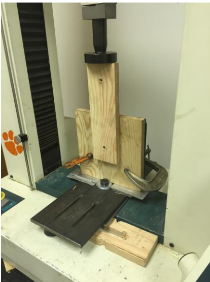
Figure 7: Screw Shear Test Setup
