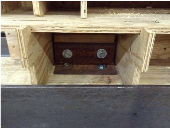
Figure 15: Angle Connection Wall to Frame
