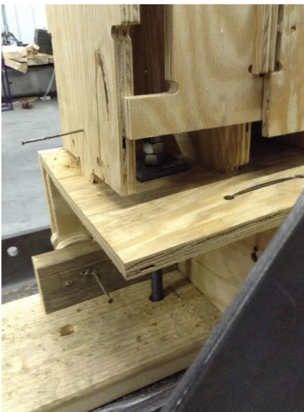
Figure 17: \frac{3}{4} " Vertical Hold Downs Rods
