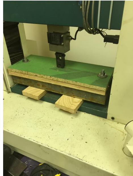
Figure 11: Screw Withdrawal Test Setup
