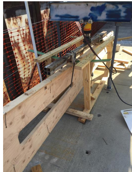
Figure 25: Rafter Test Setup
