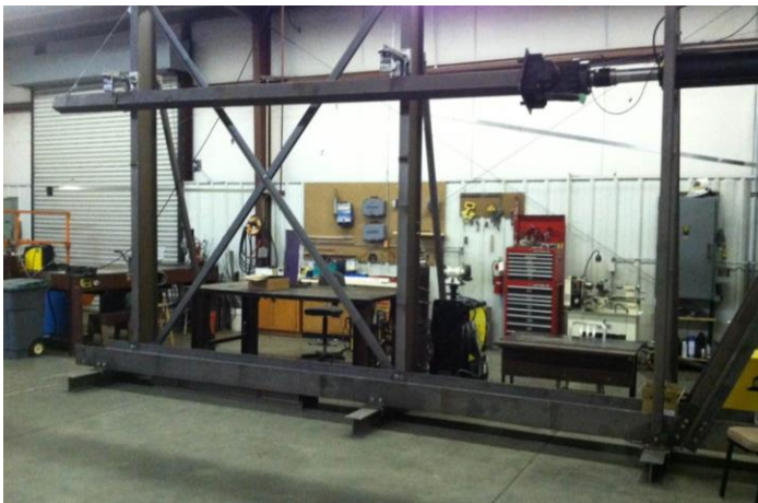
Figure 14: Shear Wall Testing Frame
