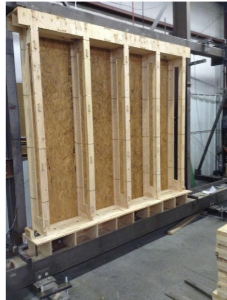
Figure 13: Wall Loaded into Shear Wall Testing Frame
