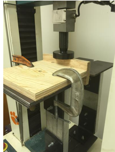
Figure 5: Shear Tab Test Setup
