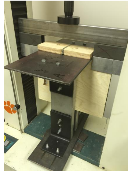
Figure 9: Cable Tie Test Setup
