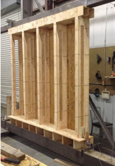
Figure 18: Wall Assembly and HSS Attachment
