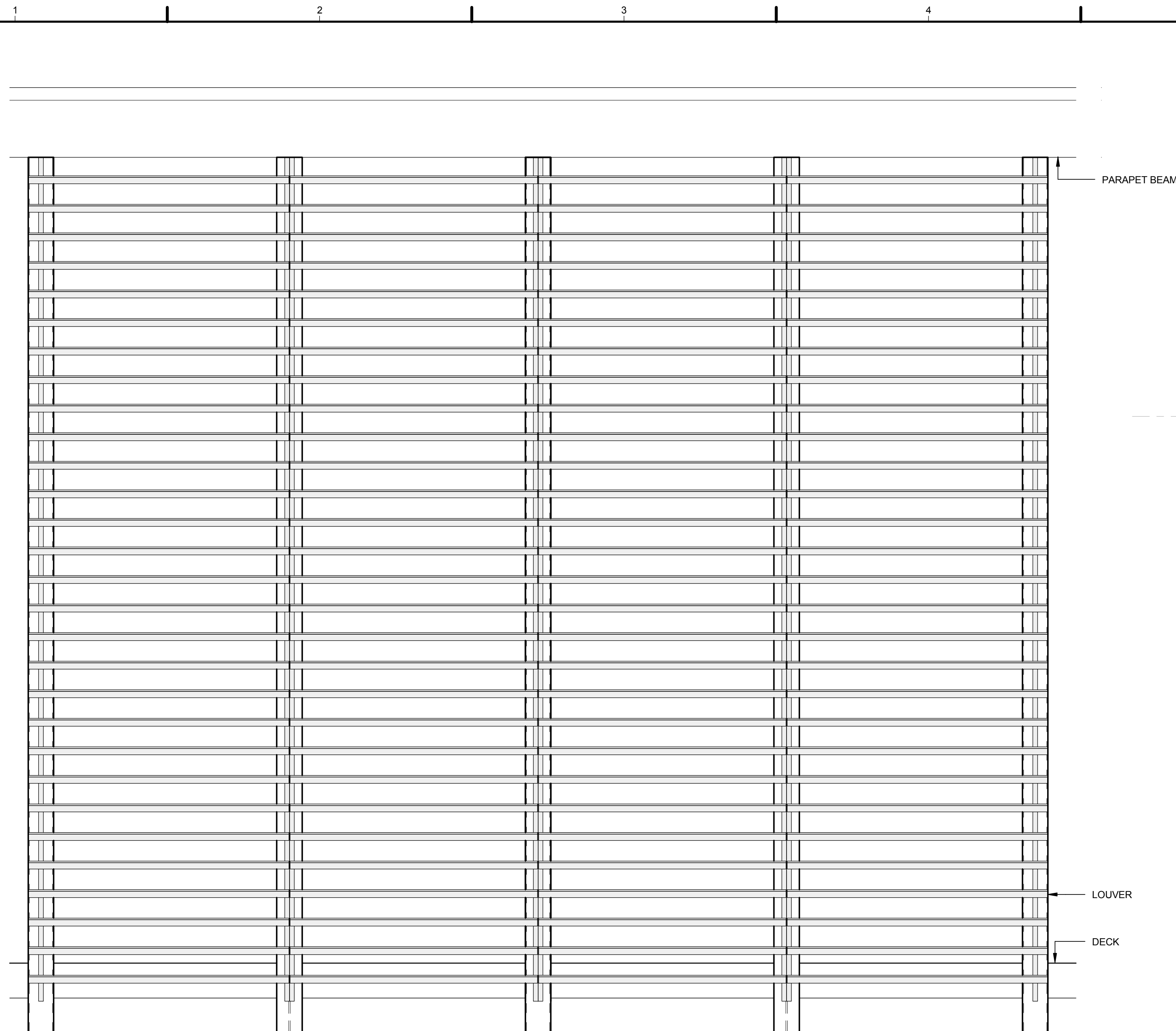
B1 LOUVER TYP. BAY ELEVATION 1" = 1'-0"
