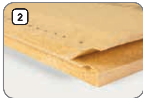
GUTEX Ultratherm® A strong rain-tight sarking board with a single-ply construction and a homogenous cross-section, this product's high U-value makes it very suitable for new roofs and roof refurbishment.
