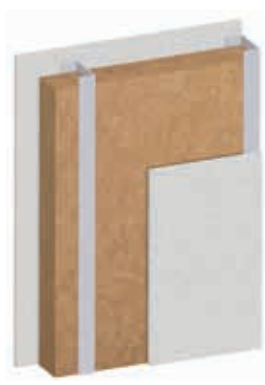
Lightweight partition walls with metal studs and GUTEX Thermofibre®/ GUTEX Thermoflex®/ GUTEX Thermosafe-homogen®
