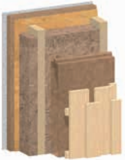
Vented facade assembly over framed construction with GUTEX Thermofibre ® , GUTEX Thermoflex ® and GUTEX Multitherm ® behind a wooden facade
