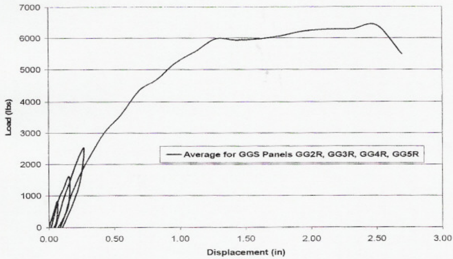
Figure No. III-5: Average Results for Racking Load vs. Net Deflection for 8' GGS-GGS Panels
