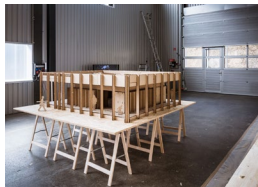
[8] 1/7-scale mockup of the modular construction: testing of the connections and logistic planning
