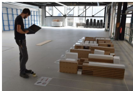
[8] 1/7-scale mockup of the modular construction: testing of the connections and logistic planning
