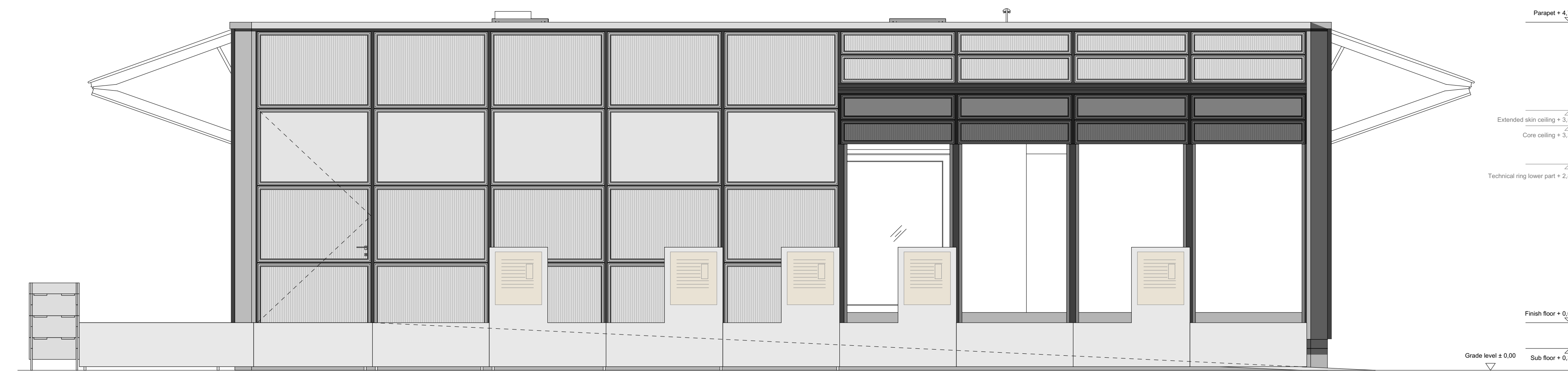
C1 NORTH ELEVATION - OPEN SKIN DOORS CONFIGURATION
