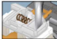
Blocked Insertion: Insertion of object in any one side will not open shutters.
