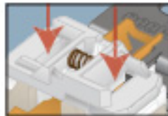
Successful Insertion: Insertion of two-bladed plug at the same time will open shutters.
