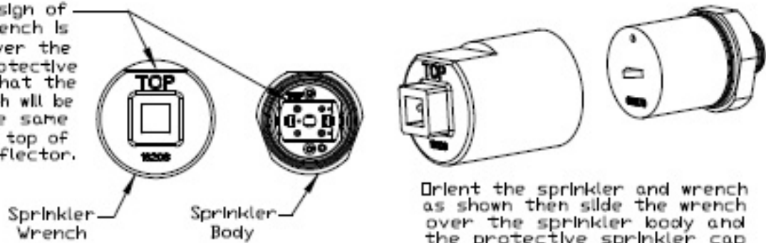
Figure 2: Sprinkler VK480 Installation and Correct Use of Wrench
