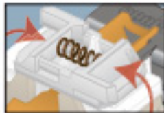
TR Receptacle Internal Components: Receptacle openings are restricted by internal shutters (show above).
