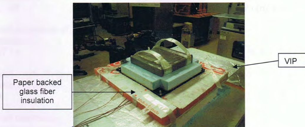
Figure 1 – Specimen in the Heat Flow Meter
