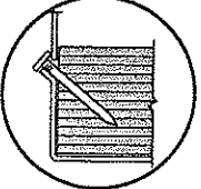
LBV features positive angle nailing, no web stiffeners are required
