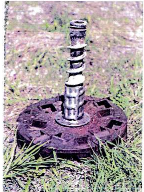
Anchor plate fixed with centring aid
