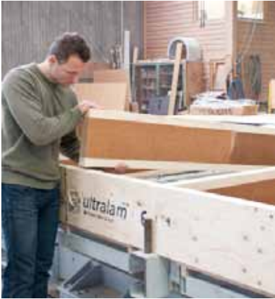
Factory produced wall cassettes with STEICO LVL R and STEICOwall.
