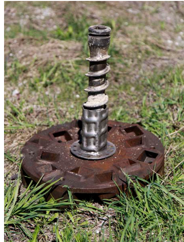
Anchor plate fixed with centring aid
