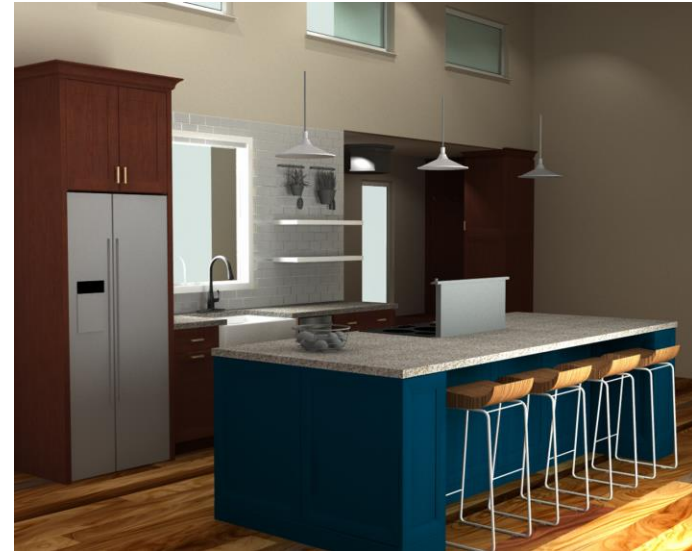
Figure 4: Clerestory Windows used for Daylighting above the Kitchen
