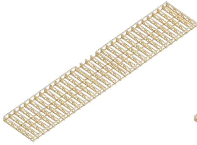
Step 1: Floor Truss Assembly
