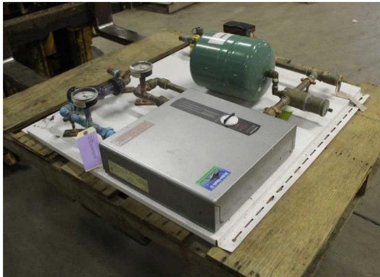
Figure 4: Electric Back-up Boiler System (Hydro Shark)
