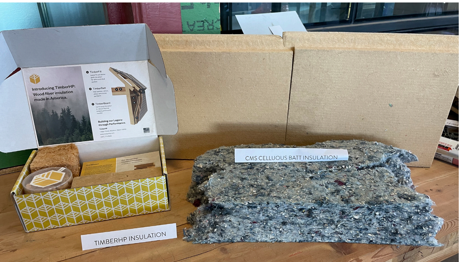
Haven Studio, photograph of TimberHP Insulation and EcoCell Cellulose Insulation.
